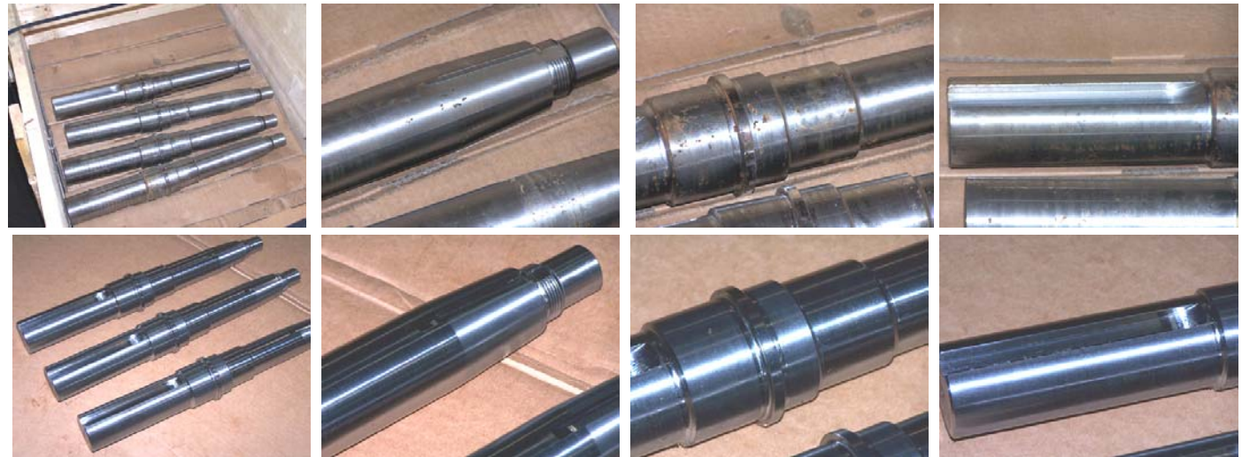
Before /After Rust Removal
